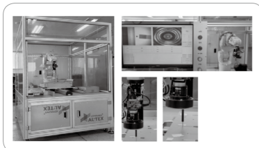
[Tap Hole Vision Inspection Equipment]
